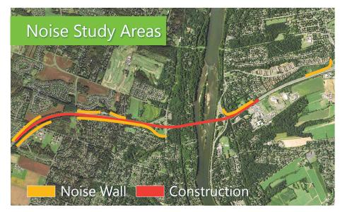
The Delaware River Joint Toll Bridge Commission contracted for a Preliminary Engineering Noise Analysis to assess the effects of traffic noise from the Scudder Falls Bridge Replacement Project. Based on that study, the project includes a series of noise walls to be constructed adjacent to locations identified as likely to have impacts. Additional noise readings were recently collected.
